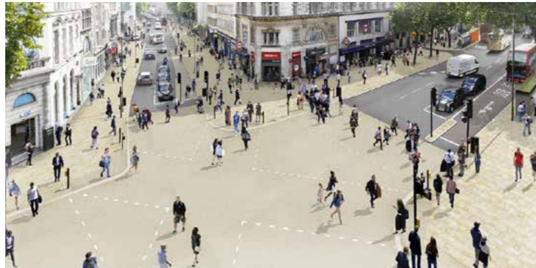
The LDA proposal for LB Camden 2015 includes the pavement widening and new diagonal 'super crossing' that are currently being implemented as part of the Holborn safety scheme.
