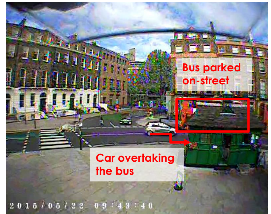
Camera No.9 – Bus stand forcing car to overtake on the opposing lane.
